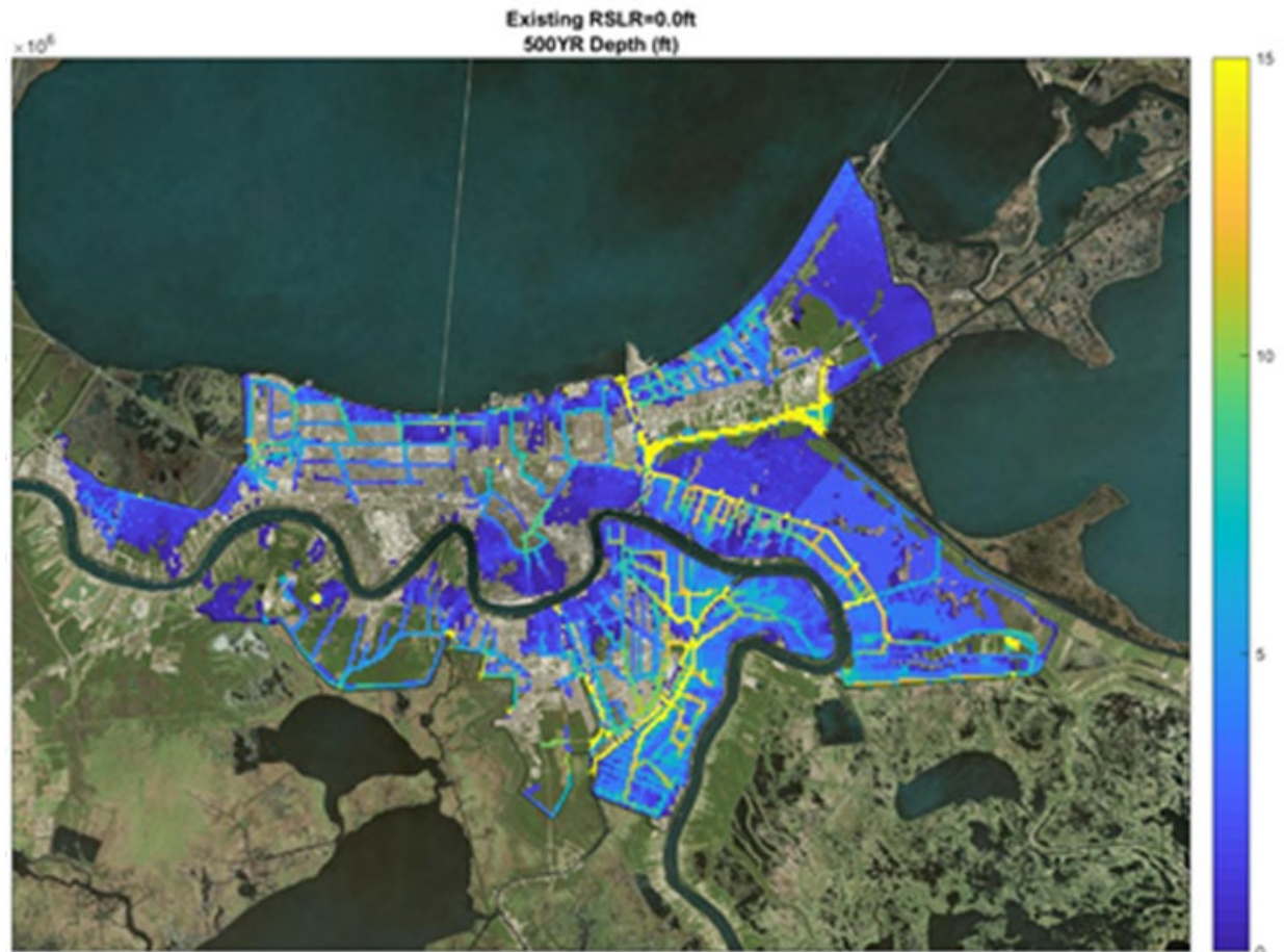
Figure 3-3. 0.2% AEP Peak Depths (ft.) for Existing Conditions
