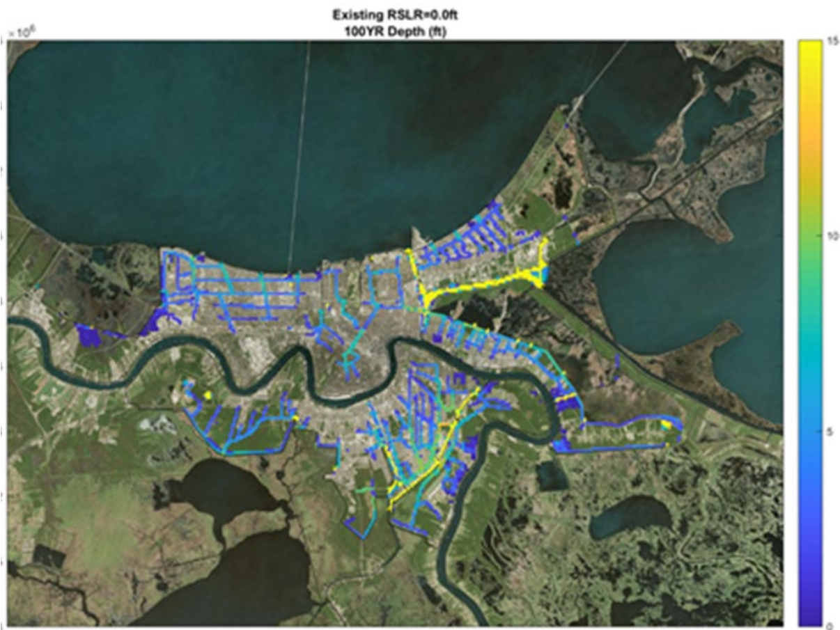
Figure 3-2. 1% AEP Peak Depths (ft.) for Existing Conditions
