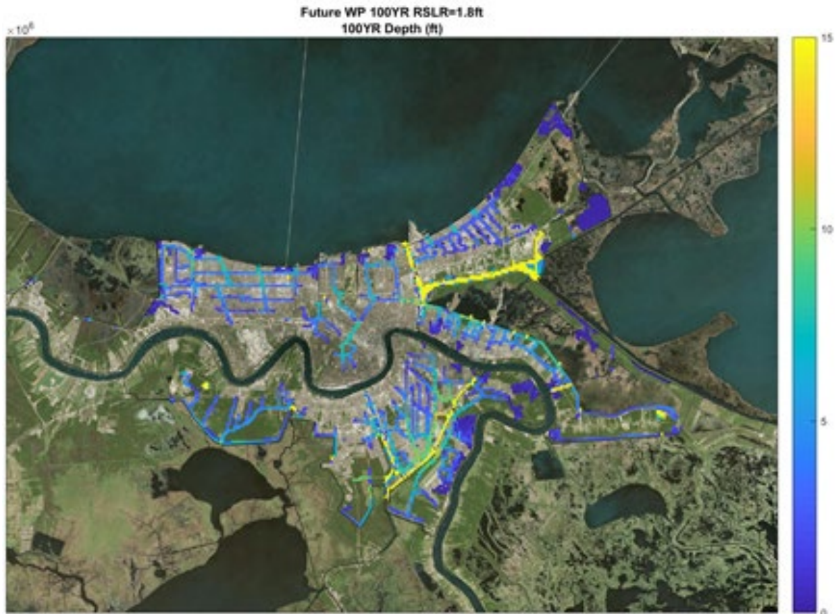
Figure 9-5. Residual Flooding for the 1% AEP Event with Full Performance of the TSP
